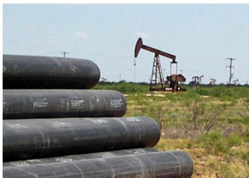
A properly marked HDPE pipe includes relevant standards on the pipe's printline to identify piping materials that meet specific standards, and confirms that the pipe is suitable for its intended purpose. It is also recommended that purchasers review the pipe manufacturer's certification reports along with physical plant inspections or independent third-party validation.
